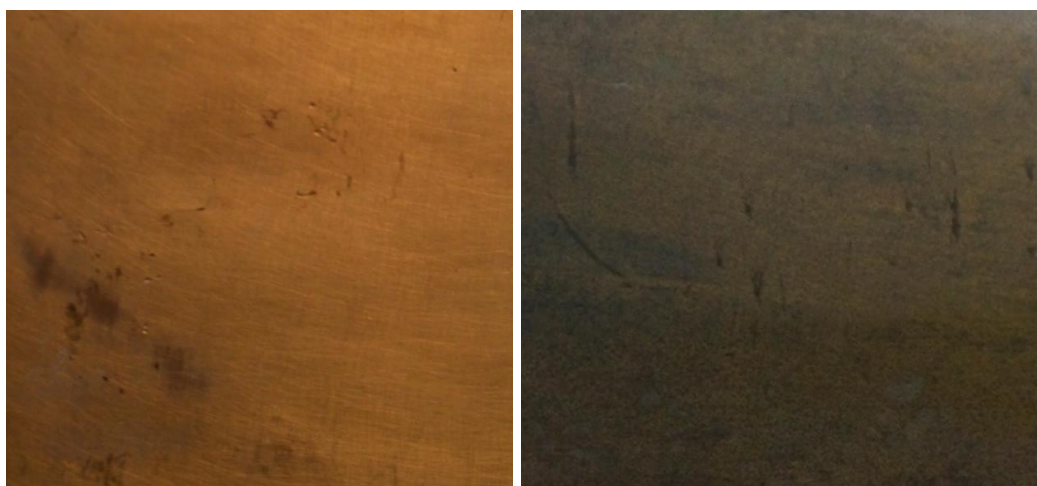
Figure 25 Magnified image of the uneven surface of a coupon showing defects and micro holes (left), compared with the uneven surface of an actual contemporary copper-alloy artifact (right).
