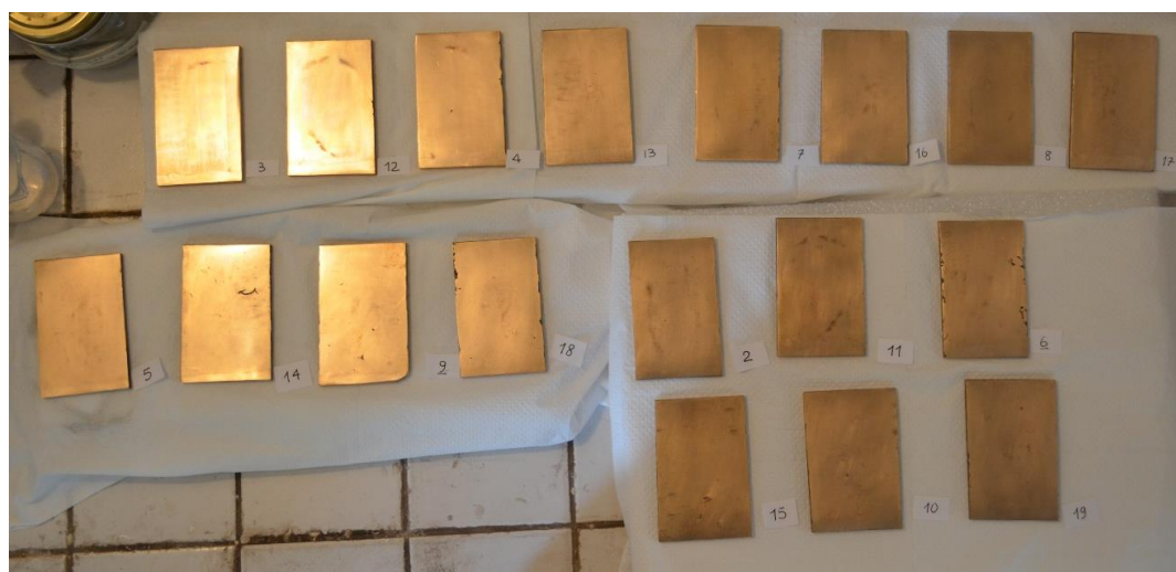
Figure 26 Bronze coupons after coating.
