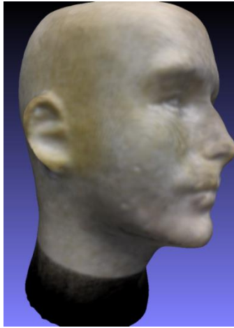
Figure 21: 3D surface reconstruction of a point cloud consisting of 45 consecutive aligned point clouds (see Figure 14) using the Poisson Surface Reconstruction algorithm [20].
