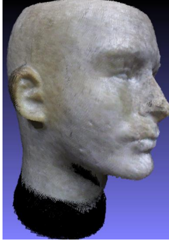
Figure 14: The final point cloud consisting of 45 consecutive point clouds aligned in the same coordinate system.
